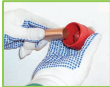
Removing internal burrs: A de-burring or reamer to be used to remove internal burrs.
